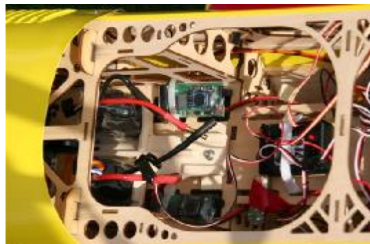
Akkubrett, Doppeltes BEC & EagleTree Telemetrie
